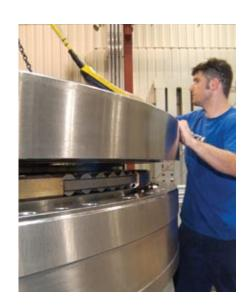
Rotek Incorporated offers a diverse line of large-diameter slewing rings: ball and roller types in single-row and multiple-row configurations; with integral internal or external gearing, or gearless models; diameters from 12 inches to 50 feet; in a wide range of load capacities, materials, and seal composites.
